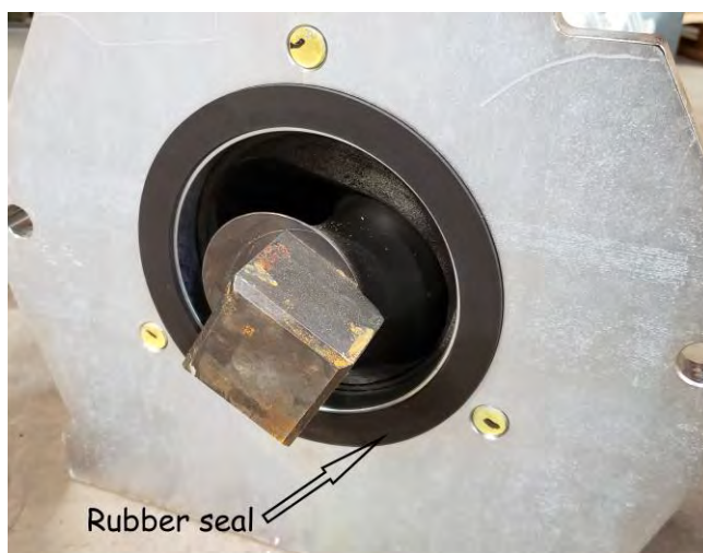
New seal fitted in position – 2L8 rotor shown
