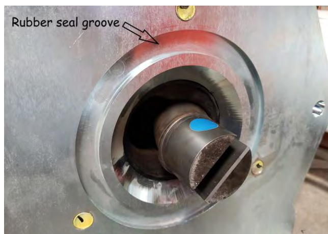
Cleaned seal groove – 6012 Rotor shown
